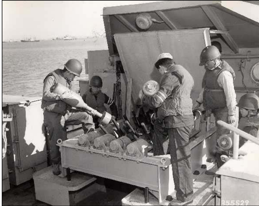
The Hedgehog was the first stand-off shipboard anti-submarine weapon. The warhead was propelled up to 250 yards by an impulse charge of smokeless powder. The explosive charge consisted of 30 pounds of TNT, or 35 pounds of Torpex. The hedgehogs were loaded on cylindrical bars called spigots, shown here, with six hogs in each cradle, and four cradles in the firing projector.
