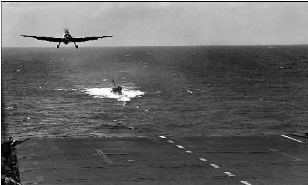
U-505 under tow by the escort carrier USS Guadalcanal in late June 1944, bound for Port Royal in Bermuda. The freewheeling of the sub's twin screws generated electricity aboard the sub, crucial to its control. A TBM Avenger patrol bomber is coming in to land on the Guadalcanal's flight deck.
