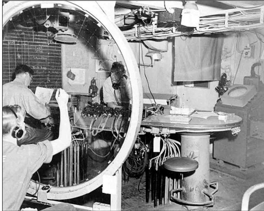
The nerve center of the Hunter-Killer ASW task groups was the Combat Information Center, or CIC, aboard the flagship jeep carrier, shown here. Position fixes were noted with wax pencils on the transparent circular plotting board, at left. This assumed the position of the carrier at the center and used the ship's radars for ranging to potential targets, based on information fed from its own aircraft and screening escorts. Discovering an enemy submarine within the perimeter of the hunter killer task group was a terrible failing, but that is the situation that presented itself to Task Group 22.3 on June 4, 1944.
